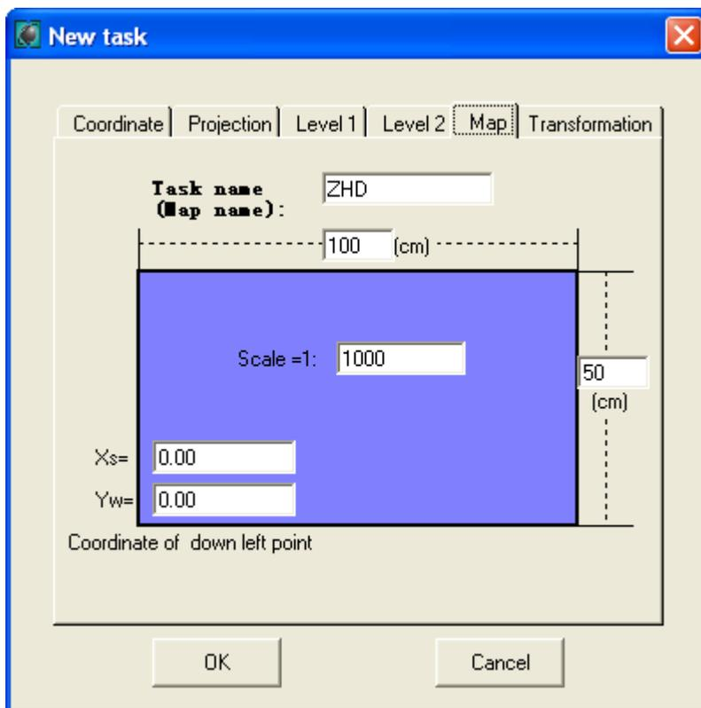
"Map" Note: A new frame must cover all of the working area; the southwest point to be correct is very important.
