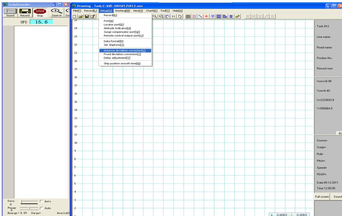
Just as we suggest locating the GPS receiver (or GPS antenna if you use a split GPS receiver) on the right above of the transducer, so here below we can make the settings much easier: (+x is the heading)
