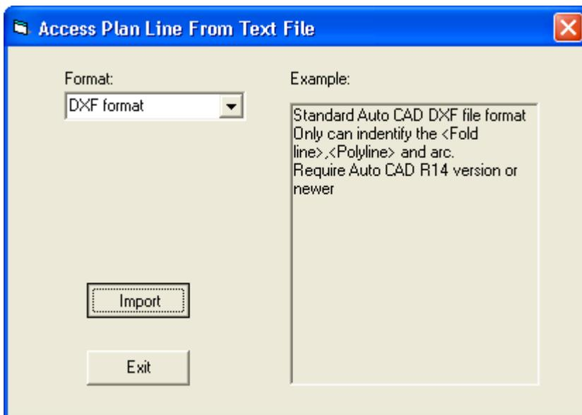
Then choose the DXF file which must be with the same coordinate system and surveying area with the project in this echo sounder surveying software project.
