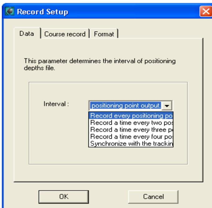
Furthermore, you can set the collection interval for the positioning data, usually we choose the below two ways (for the interval, usually if in a very small area such as below 1km\*1km, you can set 10 meters as the interval; if in about 2km\*3 km surveying area, you can set 20 meters sampling; if even larger to be 5km or more as the side length, usually we set 50 meters. But this depends on the surveyors requirements):
