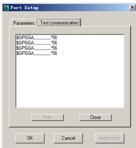
Once being successful in “Port Setup”, enter “Data Format” after pressing “Setup”
