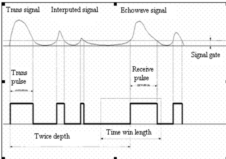
Figure 1-2 Tracking technique of the Time Gate
