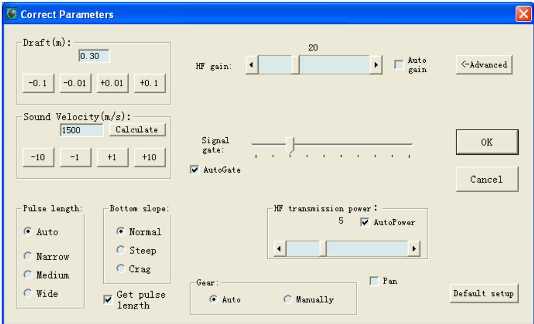
**Figure 2-11 Parameters and environment configuration**
