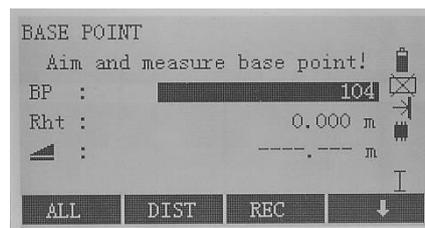
It is possible to measure the height starting from the prism position or from the base point.
