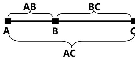
1. Select a point B on the approximately horizontal line AC with about 100 meters long. Measure the distances of lines AB, AC and BC.
