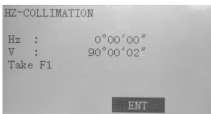
Aim at the cross-hair of collimator at telescope left, and it'll display the horizontal and vertical angles.
