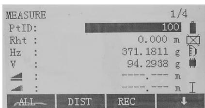
Sight the 2nd target. The displayed Hz value is the included angle between two points.
