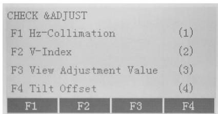
Then, F1 "Hz-Collimation" to access collimation error process.
