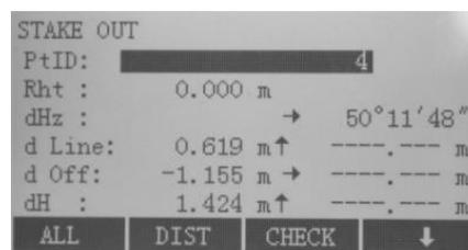
Move the instrument, according to the indicated arrows to find the point position:
