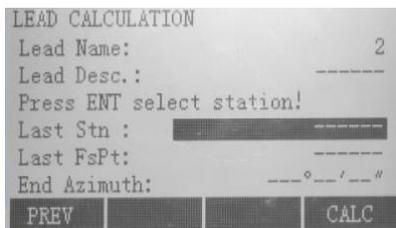
Similar with "Lead Set", when moving screen cursor to "Last Stn" and "Last FsPt", you can press [ENT] key to search the point you need or input coordinates.
