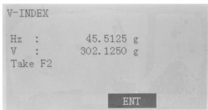
Aim at the cross-hair of collimator at telescope right, and it'll display the horizontal and vertical angles. Press F3[ENT] to take face II.
