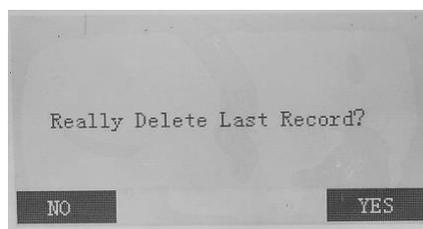
**NOTE:** Deleting, the last record is not reversible! Only records which were recorded in "Surveying" or in "Measuring" can be deleted.
