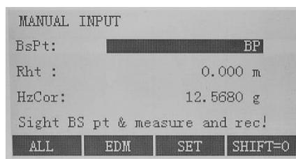
2. Coordinate orientation: press [F2] key. Orientation coordinates can be either obtained from the internal memory or entered manually.
