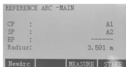
Then, decide to measure or stake out. Press F3[MEASURE] key to activate Line & Offset measuring or press F4[STAKE] key to start the application to stake out. Using F1[NewArc] it is possible to change the arc.
