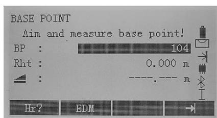
In the remote height main page press F4[ ↓ ] key to scroll the softkeys. Then, F1[Hr?] key to start the program that determines an unknown prism height.
