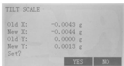
If both correction constant are in the range, press F3[YES] to renew the correction angle, or press F4[NO] to give up this adjustment,
