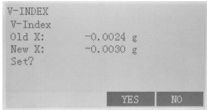
The software will calculate the new collimation error and vertical index error automatically. Press F3[YES] to renew the correction or press F4[NO] to give up this adjustment.
