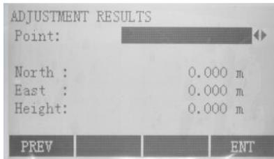
Press F2[**MORE**] to check “calculation results”, especially coordinates of each lead point after computing.
