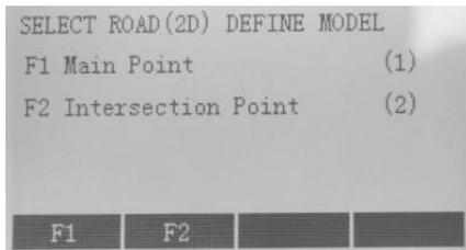
Press F2 "Road(2D) Define Data". This application is used to describe and determine road centerlines. As shown, there are two models available for Road(2D) definition: "Main Point" and "Intersection Point".
