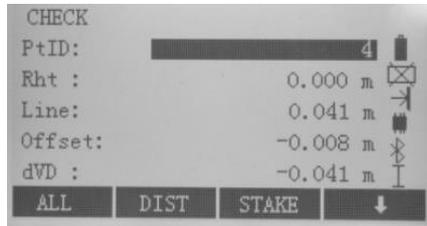
Press F3[CHECK]; the display will show you the line offset (**Line**), the transversal offset (**Offset**) and the height (**dVD**) of a measured point in relation to the line.
