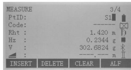
**[INSERT]:** If a character was skipped (e.g. 13 instead of 123), you can insert it later. Place cursor on "1", insert an empty character on the right of "1" pressing F1[INSERT] key. Input the new character "2" and confirm input.
