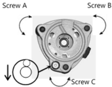
Move the bubble to the center of the circle by turning screw C.
