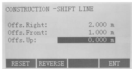
Press F4[ ↓ ] and F3[MAxis] keys to input values for shifting the line.
