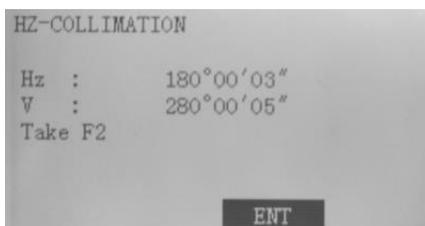
Aim at the cross-hair of collimator at telescope right, and it'll display the horizontal and vertical angles
