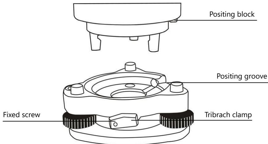
**NOTE:** Fix the tribrach clamp: if the instrument doesn't need assembly or disassembly from tribrach frequently, it is necessary to fix the tribrach clamp by fixed screw to avoid the disassembly by accident.
