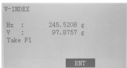
Aim at the cross-hair of collimator at telescope left, and it'll display the horizontal and vertical angles. Press F3[ENT] to take face I.
