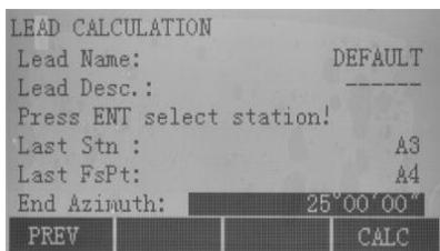
**NOTE:** If the lead belongs to branch traverse, directly press F4[CALC] key to compute coordinates of each lead point of branch traverse.
