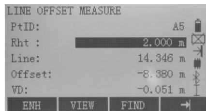
The calculated height difference is relative to the selected reference height (**VD**).
