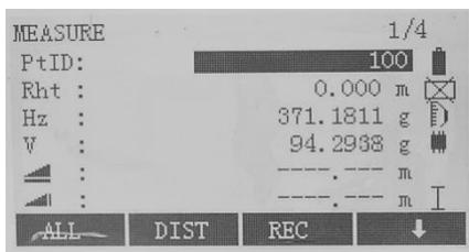
Aim at the target and press F1[ALL] or F2[DIST] to start measuring distance.
