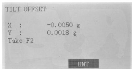
"Take F2" is displayed. Rotate the top of instrument 180°/200gon. Wait a few seconds for the display to stabilize, then press F3[ENT].
