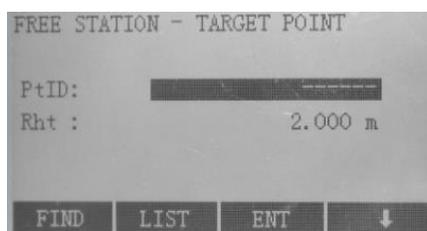
Input of the target ID (PtID) and the reflector height (Rht). It is also possible to select a point from the memory through F1[FIND] or F2[LIST] or to input coordinates pressing F4[↓] and F1[ENH]. Press F3[ENT].
