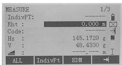
Press F4[ ↓ ] three times, until when the [IndivPt] softkey appears in the black bar at the bottom of the display. Press it to switch between individual and current point ID. With this function, it is possible to shift from continuous point collection to individual point collection. Edit the individual point ID and press F1[ALL] key to measure and record it.
