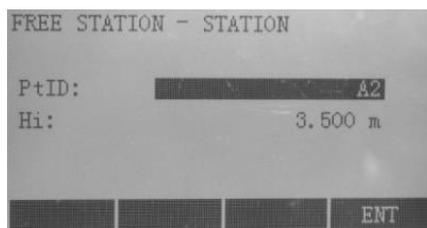
Input of the name of the station (PtID) and the height of the instrument (Hi). Press F4[ENT].
