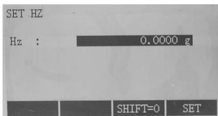
Use the F3[SHIFT=0] key to set the 1st target as 0° in the measure mode.
