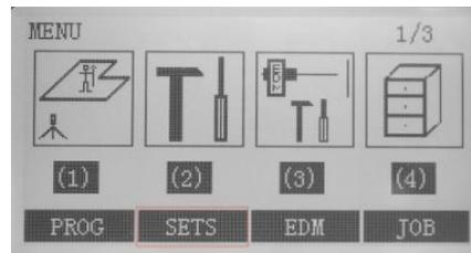
Select [SETS] item, where relevant parameters can be set. Press {PAGE} key to scroll all the commands and use ◀/▶ keys to set the options.
