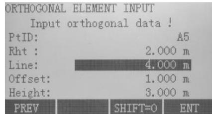
Press [ENT] to confirm data entry and start calculation. The orthogonal stakeout menu will be shown.
