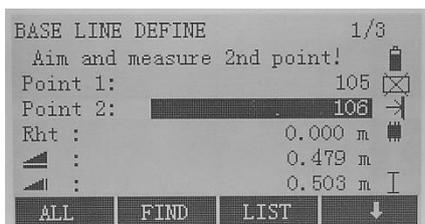
The base line is determined by two base points that can be defined in three ways:
