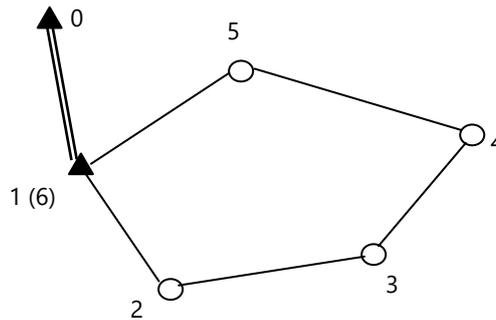
**NOTE:** As to this type of traverse measuring, the last survey station must be measured again on where point 1 is, but occupied point can't be set to point 1, otherwise this operation will make measurements of the first survey station covered. For example, occupied point of the last survey station can be set to point 6 whose coordinate inputting is the same as point 1's.
