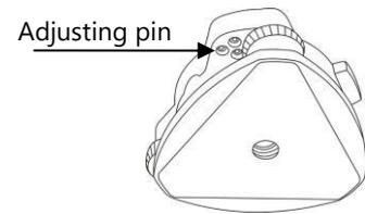
**NOTE:** Be careful when adjusting the three screws, and the tightening tension is identical for them.
