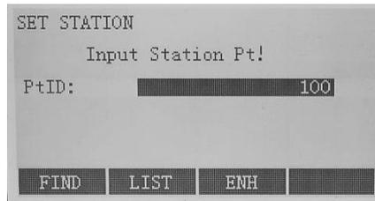
Press [F2] to set the station. Afterwards choose either of the two following methods to complete the application of setting station.
