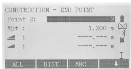
Automatically, stake out display is shown: here you can search or enter points (in the same way as in the previous step) to stake out.
