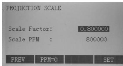
**Scale Factor:** Measured values and coordinates are corrected with the PPM parameter. Limit value: 0.50 to 1.999999;
