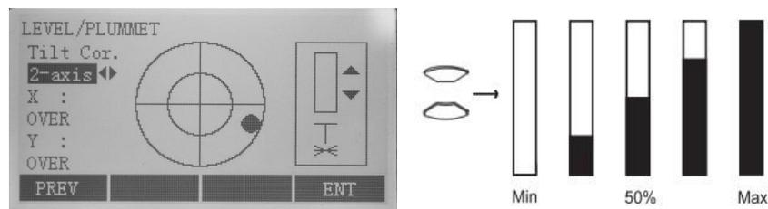
Press the {FUNC} key, and then click F1 or (1) keys to enter the display shown in the upper figure. With pressing ▲/▼ keys you can turn on or off laser plummet and set it as four levels of brightness. Thus, that laser emitting downwards can be seen.
