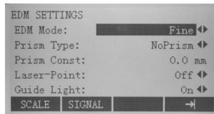
**EDM Mode:** It possesses three sorts of modes (Quick, Track and Fine) for availability. Worth noting that along with selected measuring mode the selections of prism types are different.
