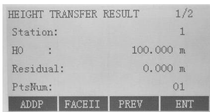
The calculated instrument height "H0" is displayed. Press {PAGE} key to see the calculated coordinates and other results. Select:
