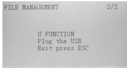
Conveniently, plug flash disk into the USB interface for data sending and selecting. By USB connection you can see the internal memory of the Total Station like a hard disk. The internal structure is of following type:
