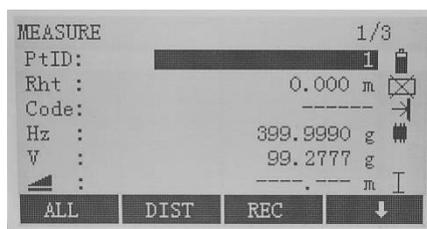
Input PtID, reflector height (Rht) and codes if demanded. Aim to the point and press F2[DIST] to measure and F3[REC] to store the point. Otherwise it is possible to press F1[ALL] to trigger and record measurements in the same time.
