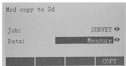
This function gives the possibility to copy a survey job from internal MSD to external SD. Please note that it is not possible to do the opposite operation. Only Survey files can be exported using this option. Select the Job and the Data which you want to copy using ◀/▶ keys and press F4[**COPY**]
