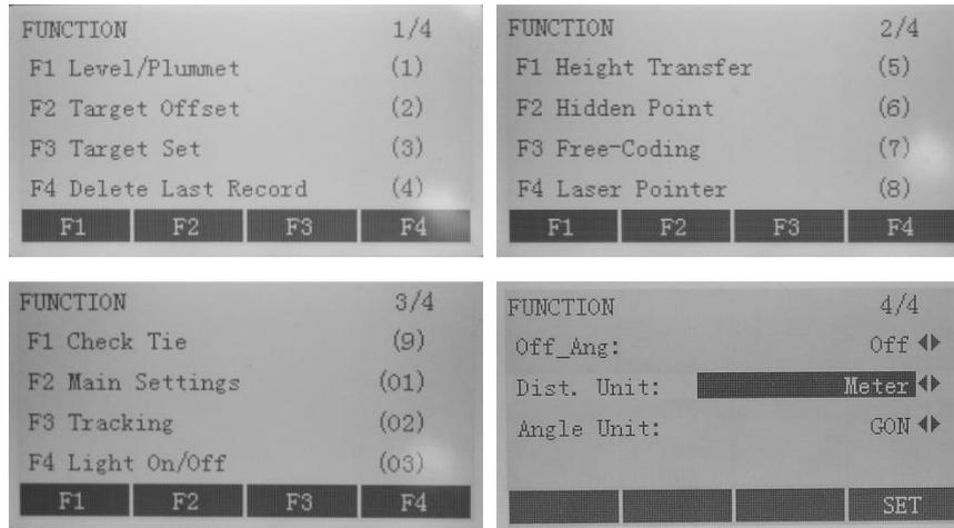
**Level/Plummet:** this function triggers the electronic bubble and enables the settings of intensity for the laser plummet (see 3.4. Centering and levelling-up).
